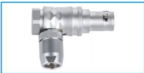
THG 90° bend plug, positioning pin (G) or positioning pin (A...M and R), cable clamp fixing and sheathed tail cover
