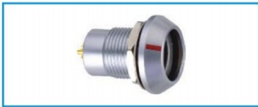
MHG fixed socket, nut secured, positioning pin (G) or positioning pin (A...M and R) watertight or vacuum-sealed (waterproof when inserted)
