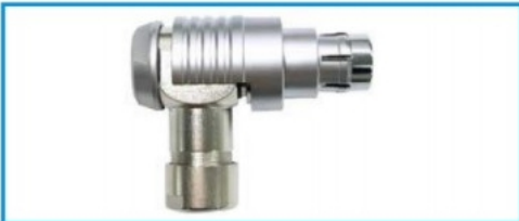
TWN 90° bend plug with semi-circular positioning plate for secure positioning, internal structure prevents cable rotation, and semi-circular metal prevents accidental insertion.
