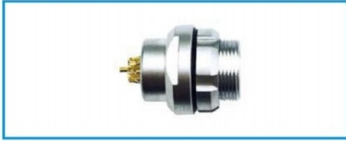
ZYN Vacuum-sealed short socket with external nut fixation and internal semi-circular metal plate positioning to prevent misinsertion, waterproof (IP68)
