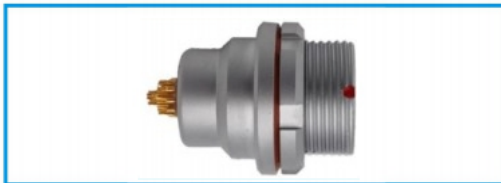
MEG fixed socket, nut secured, positioning pin (G) or positioning pin (A...F, L and R), rear panel installation, rear side encapsulation
