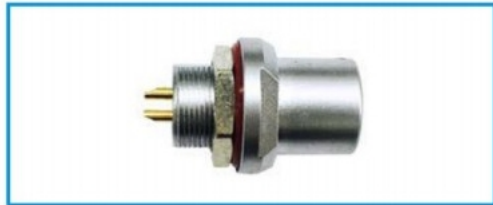
ZHN Protruding rear nut fixing socket, nut fixation (front panel installation), internal semi-circular metal plate positioning to prevent misinsertion, waterproof (IP68)
