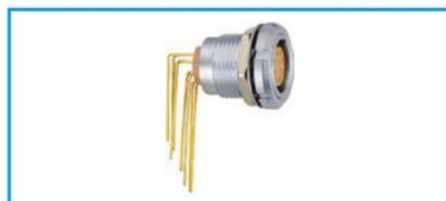
ZCG fixed socket with two nuts and positioning pin (G) or positioning pin (A.....F), suitable for 90° bent pin cores on printed circuit boards (rear panel installation)
