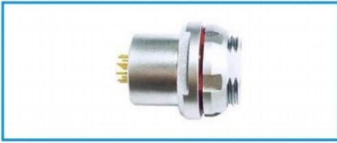
ZLN PCB board socket with external nut fixing structure and metal semicircular positioning to prevent misinsertion
