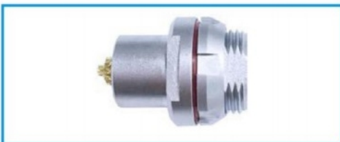
ZLN Welded socket with external nut fixing structure, metal semicircular plate positioning to prevent misinsertion
