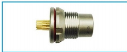
HEN Protruding tail external nut fixing socket, external nut fixing (rear panel installation), internal semi-circular metal plate positioning to prevent misinsertion, waterproof (IP68)
